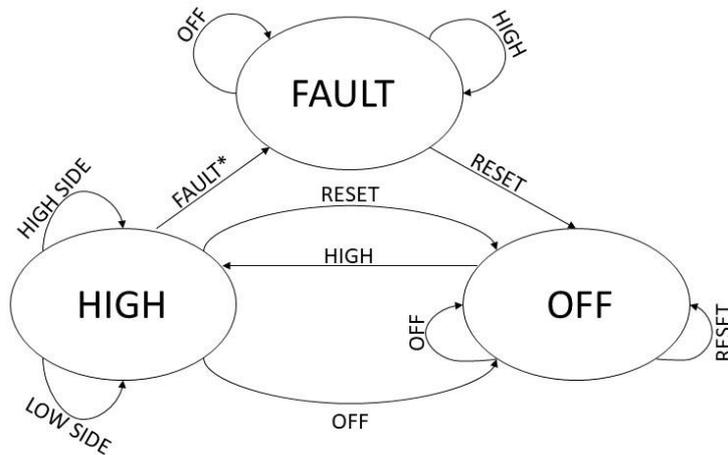
\*= If the output command is Low Side, the fault state is not detected.
