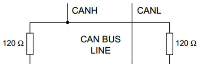
Each end of the CAN bus is terminated with 120Ω resistors in compliance with the standard to minimize signal reflections on the bus. You may need to place a 120Ω terminating resistor between CAN-L and CAN-H
